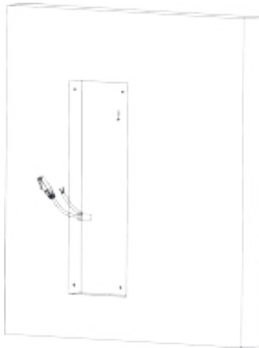
Figure 4-37 Cave the Installation Hole
