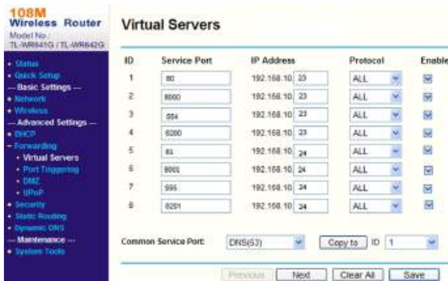
Figure 7-1 Port Mapping on Router
